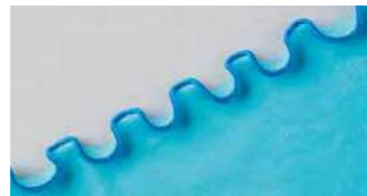
Frill 3-Thread Rolled Hem With Diff. Feed Uses 3-thread rolled hemming and the differential feed on stretch fabrics to create richly designed articles.
